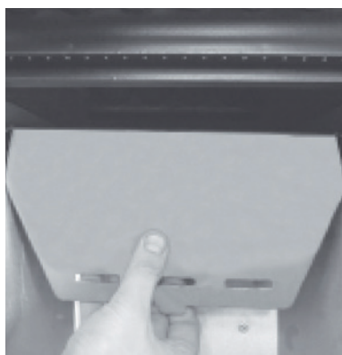
Pict. 16: Rotate the fire shield
